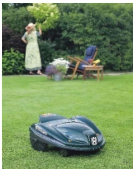
The battery-driven Husqvarna Auto Mower cuts up to 1,200 m 2 of lawn automatically, and recharges itself at a specially designed docking station.
