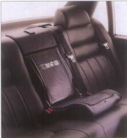
Electrolux Autoliv and Volvo have jointly developed a foldable child safety seat that's built into the back-seat center arm rest. Compatible with the standard safety belt, it's the safest place in the car for children between 3 and 10 years.
