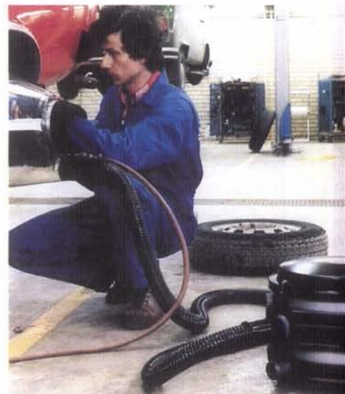
This vacuum asbestos remover is one of the new products in Euroclean's wide environmental protection line. The machine provides a better working environment in automobile repair shops.
