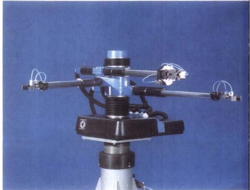
With the three-armed Electrolux MHU Junior industrial robot several machines can be served at the same time.
