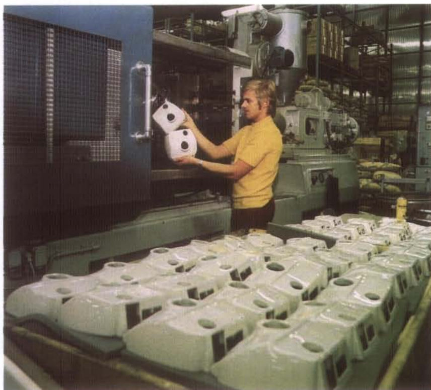
The Electrolux factory at Motala in Sweden houses one of the largest installations for injection moulding in the country. Pictured here is the manufacturing of vacuum cleaner covers made of thermoplast.
