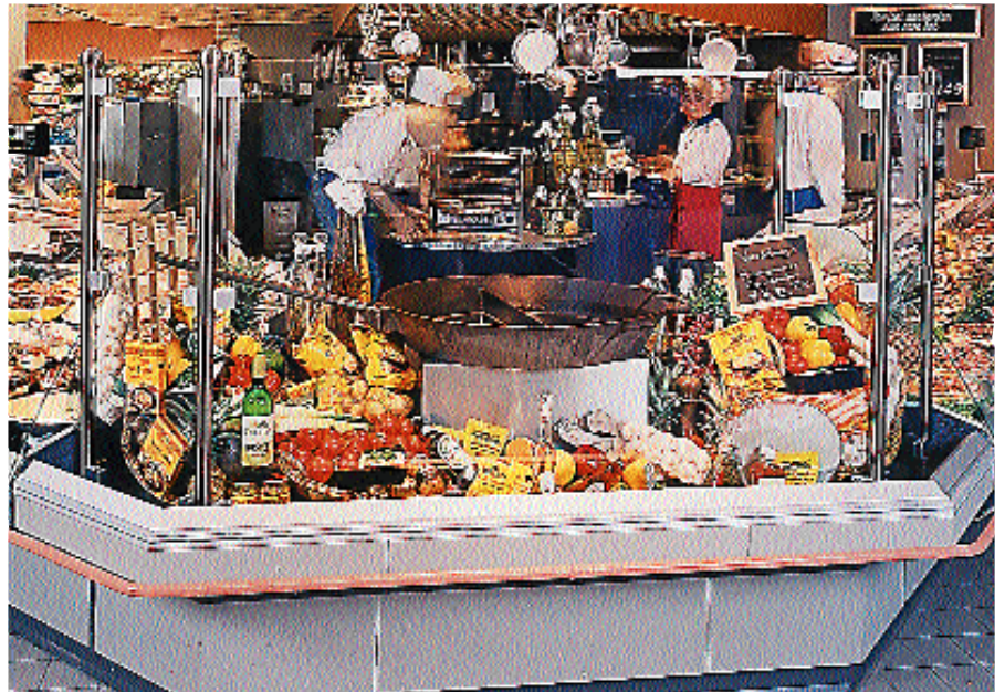
A refrigeration unit for the retail trade in the Netherlands with a CFC-free cooling system. High efficiency compressors in the cooling system reduce energy consumption by 20 percent in comparison to previous models.
