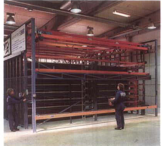
The automatic Cubinoster system for compact storage of goods with virtually any dimensions.
