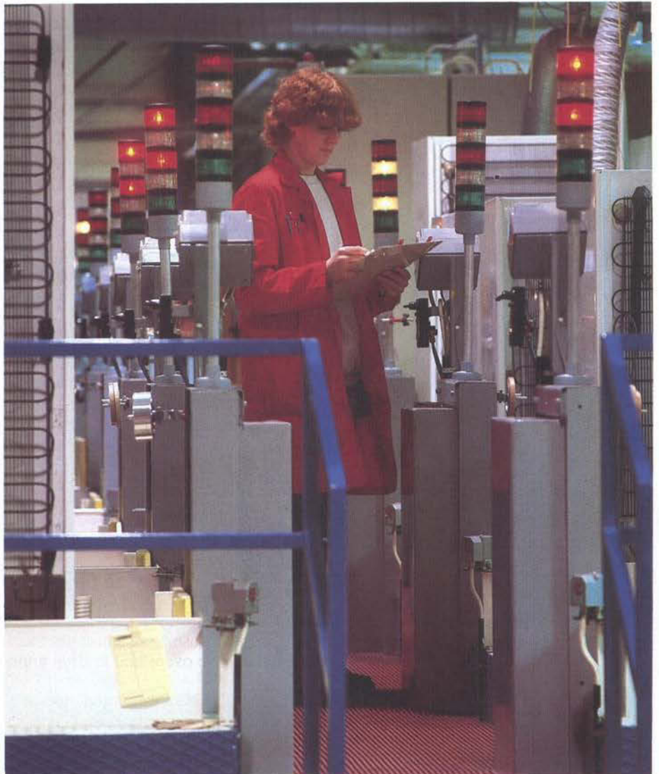
Electrolux's major quality campaign was a key feature of the activities of the various production units throughout the year. The picture shows computer controlled testing of refrigerators and freezers at the Mariestad unit.
