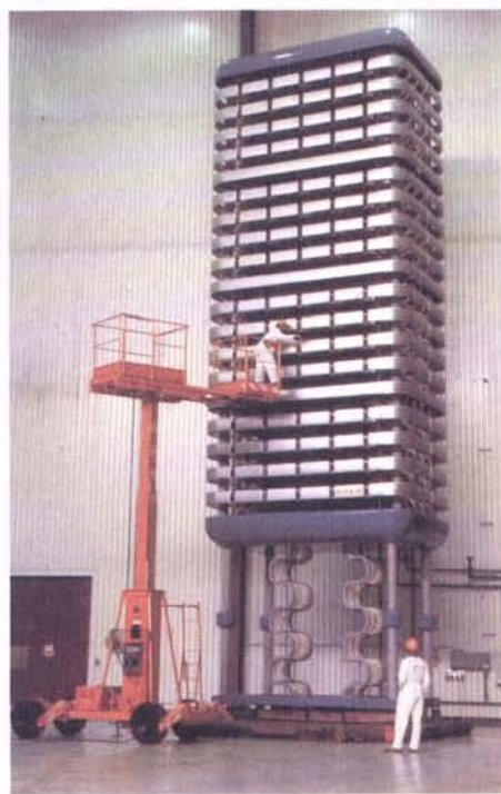
Thyristor valves for power stations incorporate PEX tube from Wirso and aluminium sections from SAPA.
