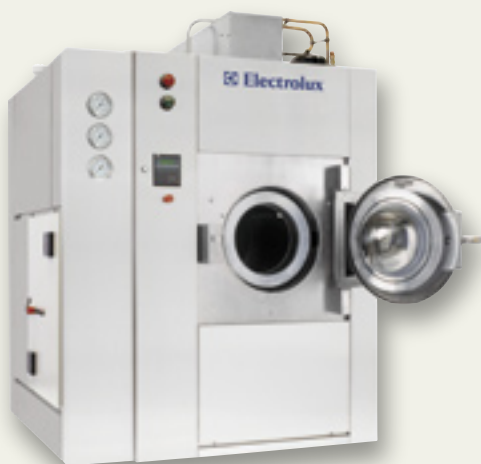
The LCO2 Dry-Cleaning System, fully commercialized in 2004, uses CO 2 instead of traditional cleaning agents to dry-clean clothes. Highly pressurized CO 2 acts as an effective, environmentally benign solvent to remove dirt. At the end of the cycle, pressure is reduced and the carbon dioxide is distilled and recaptured.
