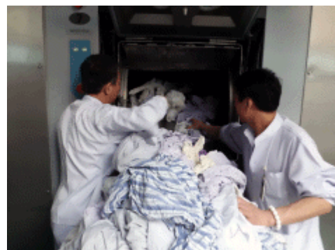
Unloading a 70 kg Pullman Barrier Washer.
