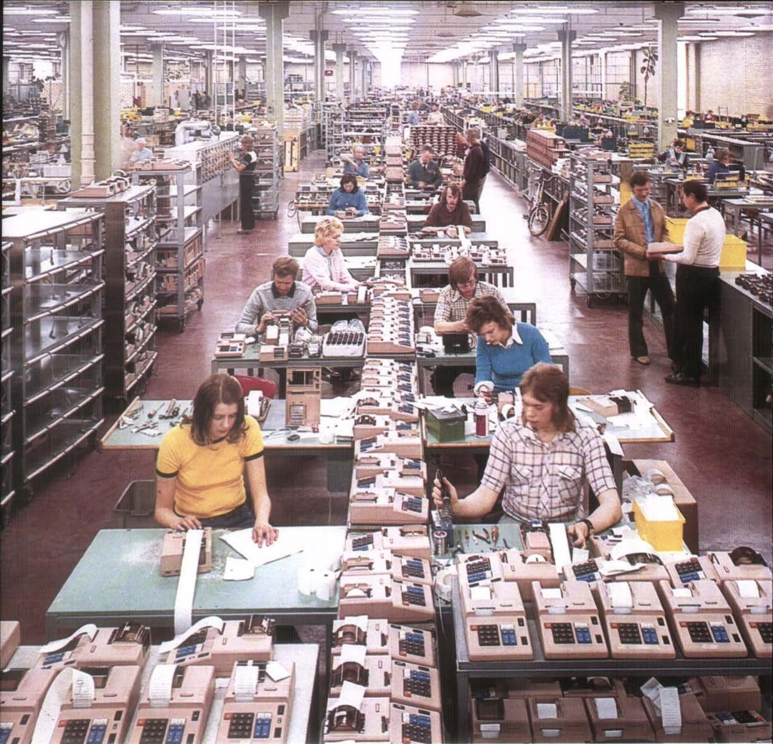
Assembly of electronic calculators with tally roll at the Örsätter factory, Åtvidaberg (Sweden). The Örsätter factory is Facit's largest and most modern factory.
