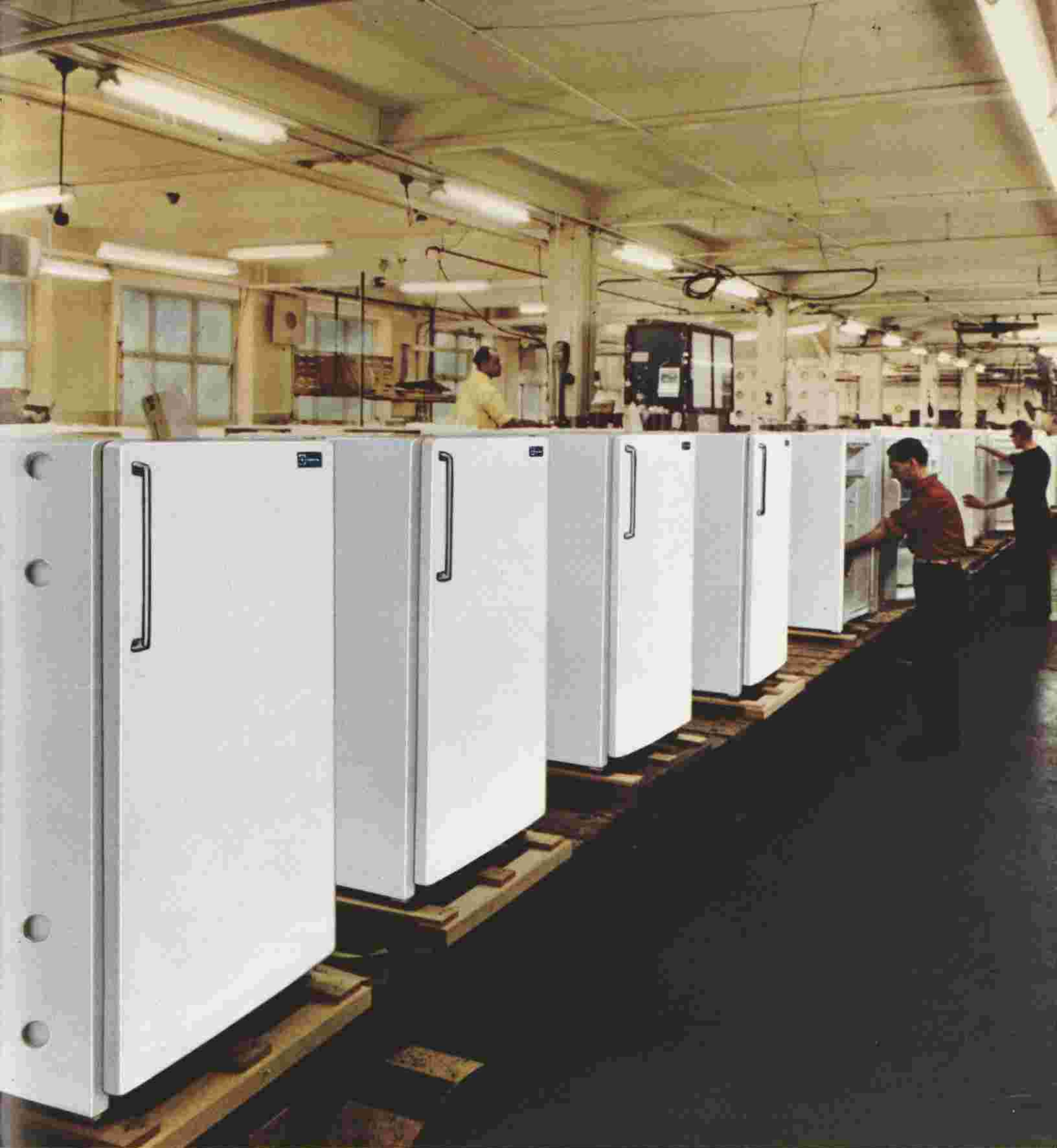
Final assembly stage of the L 43 refrigerator in the Electrolux factory at Motala. This model has a capacity of 120 litres (4.3 cu. ft.) and is operated either on gas or electricity.
